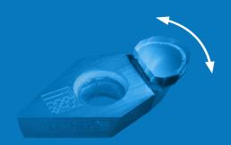
When cleaning the tool (on or off the machine) use **isopropyl alcohol or acetone** and a lint free cloth or a Q-tip. Always wipe along the front of clearance angle along the cutting edge. Paint brushes and un-filtered compressed air can hold particles that can cause damage, so are not recommended. Never drag anything from the top of the diamond over the cutting edge, as this may cause a chip-out.
