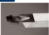
Mono-crystalline diamond tooling used in conjunction with ultraprecision, CNC machine tools are used to direct lathe specialty materials for contact lenses and intraocular lenses and/or mold inserts.
